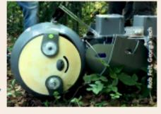
the Georgia Institute of Technology in the US will monitor animals and plant life. It is powered by solar panels and hangs on a wire suspended between two trees. The energy-efficient SlothBot moves slowly like a real sloth, collecting information such as the temperature, weather and the carbon dioxide levels of the area.
