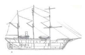
A very robust and sturdy little ship, Endurance wa designed specifically to withstand harsh polar condition: This meant that wherever possible joints and fitting were **cross-braced** and strengthened, making he extremely strong.
